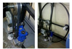
Helical geared motors, **H Series**, size 050 with 2 reduction stages, are used for twist drop towers applications, where the movement speed is not constant and with high torque peaks. These gearboxes are characterized by cast iron casing and hardened/tempered gears.
